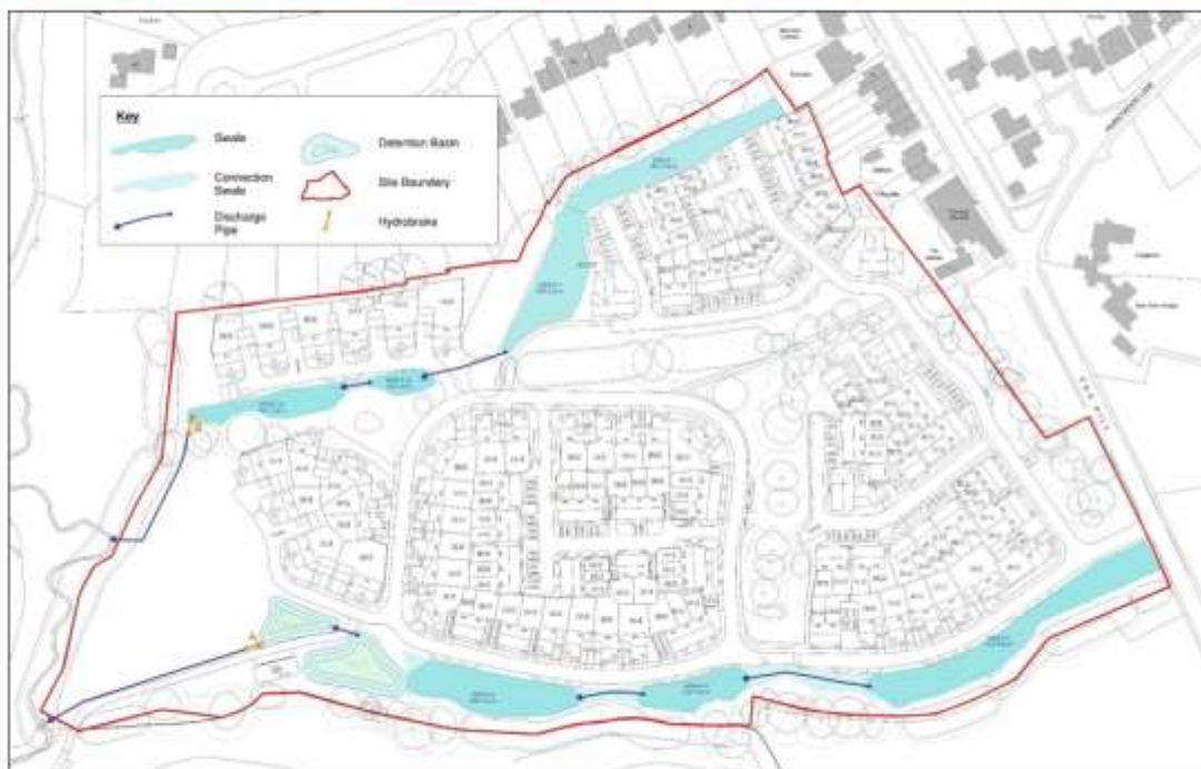
Figure 5-2 - Location of Swales and Detention Basins
